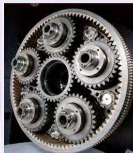
Fan Drive Gear System(FDGS)
